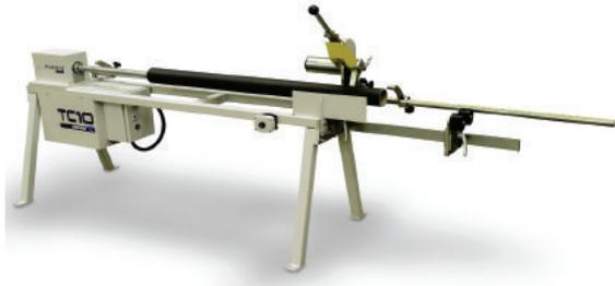
The Parkland TC10 Series R is a compact manual machine that is practical, efficient and cost effective. It produces an accurate, clean, quality cut with quick and easy change-over for multiple core diameters from 25.4mm (1") to 152.4mm (6") ID and wall thicknesses up to 20mm (3/4") on cardboard and 11mm (7/16") on plastic. For parent cores ranging from 1500mm (59") - 3000mm (118") long.
