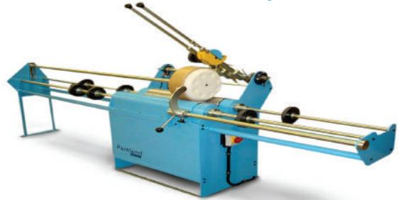
The Parkland TC20 Series R is a manual surface driven machine that is practical, efficient and cost effective and is ideal for longer and larger diameter parent cores. It produces an accurate, clean, quality cut with quick and easy change-over for multiple core diameters from 70mm (2-3/4") to 400mm (16") ID and wall thicknesses up to 13mm (1/2") on cardboard. For parent cores ranging from 1500mm (59") - 3500mm (140") long. Cutting is achieved by using a free running crush cut knife principle.
